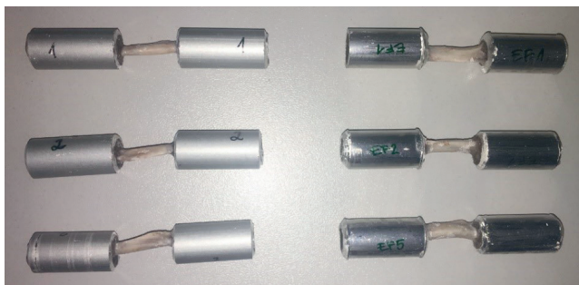
Fig. 1. Samples prepared for the four-point bending test
